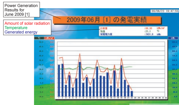
Photovoltaic power generation monitor
