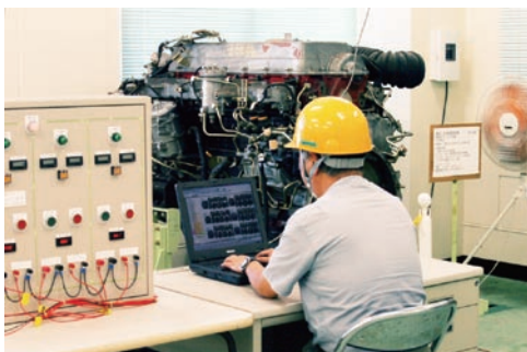
Reliability evaluation test of starters with a large truck engine
